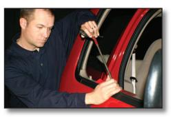
PDR works from behind the vehicle's damage; therefore, it does not require sanding, painting, or body fillers.
