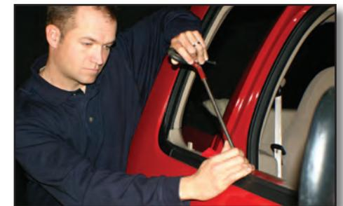
PDR works from behind the vehicle's damage; therefore, it does not require sanding, painting, or body fillers.
